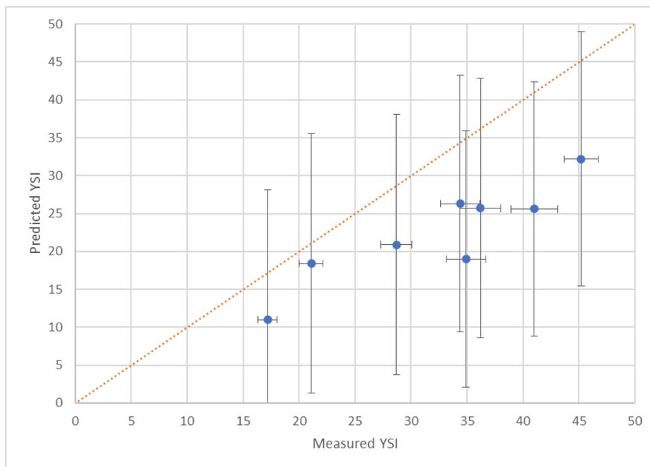
Figure 4: Predicted vs. measured YSI for the 8 studied lactones. A  $y=x$  line is shown in orange.
