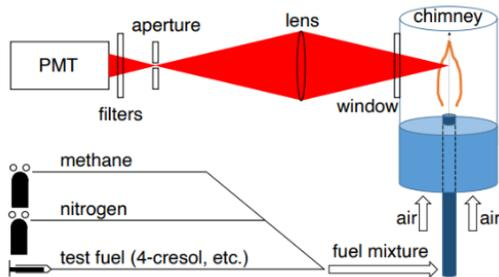
Figure 2: Yale coflow burner with LSSR setup [9]
