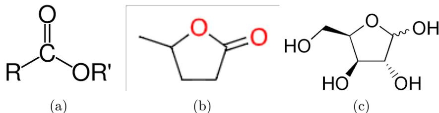
Figure 1: (a) A generalized ester structure, where R and R' denote any other functional groups. (b)  $\gamma$ -valerolactone.  $\gamma$  indicates that it has a five-membered ring, and valero indicates that it has a total of five carbons. (c) xylose in its furanose configuration, which is structurally similar to GVL
