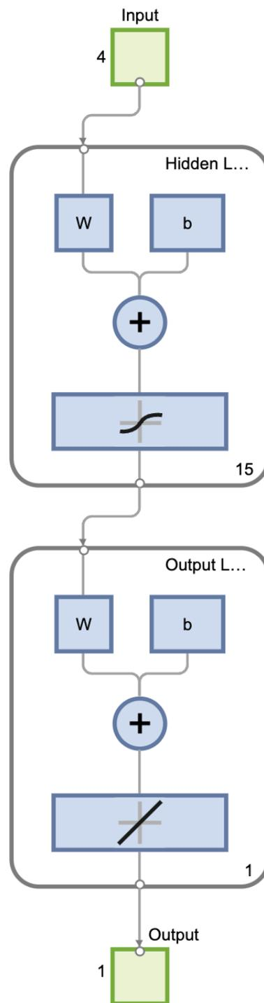
Figure 15: Overall Process of BPNN network in Matlab
