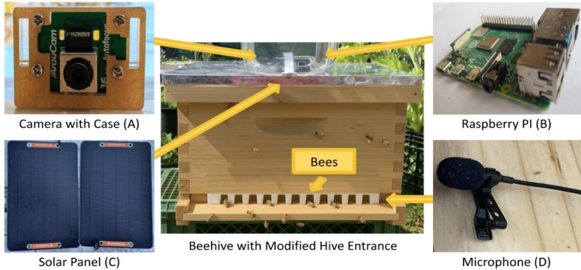
Figure 2: Automated bee monitoring system components. (A) Camera positioned above hive entrance for image capture, (B) Raspberry Pi for data transfer and system control, (C) Solar panel for a sustainable power supply, and (D) Microphone for bee sound recording.
