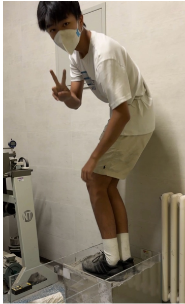
Fig. A1. Four layers of glass-fibre geogrid demonstrating sufficient capacity to support the weight of a Homo sapiens subject.
